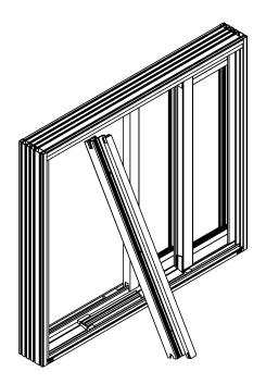
Secure second and third fixed panels with # 8- 1"screws as shown. Cover screws with mullion cover.
