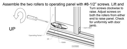
Insert panel on the operating track. Adjust height of the panel as shown. Also adjust height of rollers on second fixed panel.
