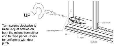
Assemble the two rollers to each operating panel with #8-1/2" screws. Lift and insert panels on the operating track. Adjust height of the panel as shown below
