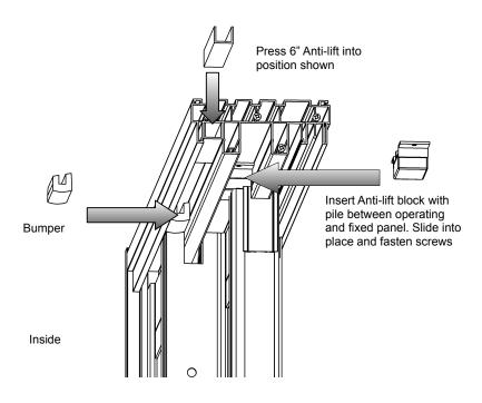
**Note:** This assembly instruction is a basic guide for qualified and experienced installers with knowledge in securely anchoring the door to the building structure. For installations in exposed areas and buildings exceeding two storeys, the anchoring requirements must be determined by a structural engineer.
