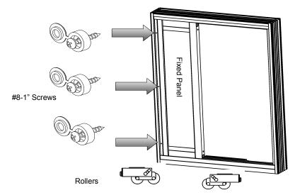
Assemble rollers on fixed panel with 2 #8 1/2" screws. Insert fixed panel into door frame. Adjust rollers (see roller adjustment). Fasten to door jamb with 3 # 8-1" screws.
