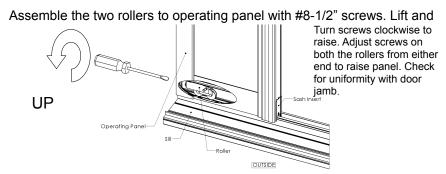
insert panel on the operating track. Adjust height of the panel as shown.
