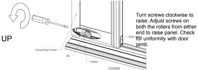
insert panel on the operating track. Adjust height of the panel as shown below
